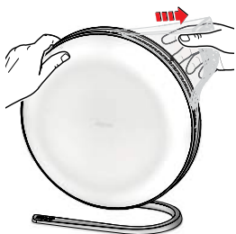
Removal of the diffuser
