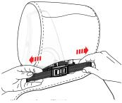
Step 5: Pull both ends of the belt out and away to tightly secure the car mount.
