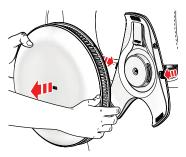
Hold the air purifier with both hands and press one or both release buttons on the car mount.
