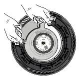
Step 3: Lift tabs to remove filter, replace with a new filter.
