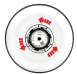
Step 2: To unlock, turn the locking ring counter clockwise.
