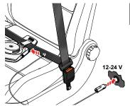
Step 3: Connect the car power adapter.
