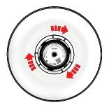
Step 4: Replace the back cover and turn clockwise to lock.
