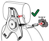
Step 6: Connect the car power adapter.
