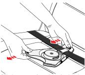
Slide the car mount forward securing the belt into the belt hook.
